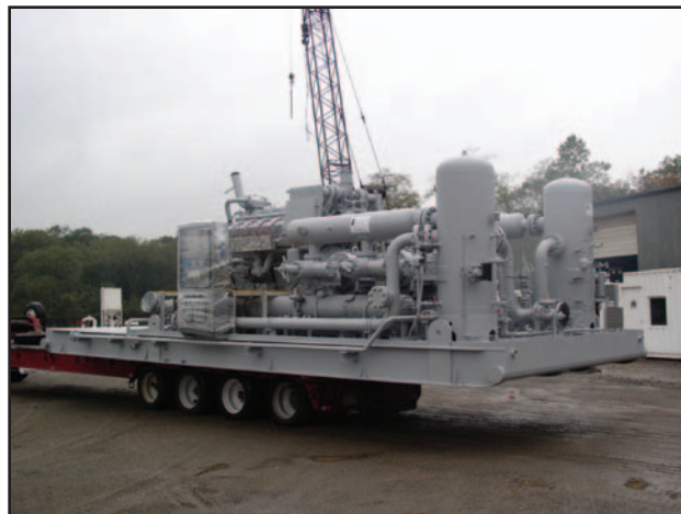
■ One month after moving into its facility, SEC received this used Waukesha 7042/Ariel JGK/4 offshore package from El Paso Natural Gas (left). In just three weeks, SEC completely remanufactured the package. It is shown on the right being loaded for shipment back to the customer.
