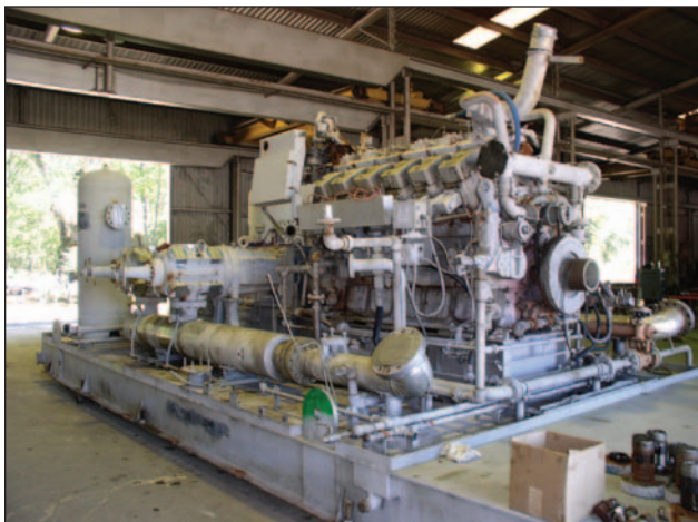
■ One month after moving into its facility, SEC received this used Waukesha 7042/Ariel JGK/4 offshore package from El Paso Natural Gas (left). In just three weeks, SEC completely remanufactured the package. It is shown on the right being loaded for shipment back to the customer.
